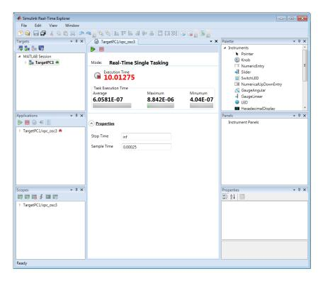
You can view the output of the real-time Scope block by connecting a monitor to your target computer.
