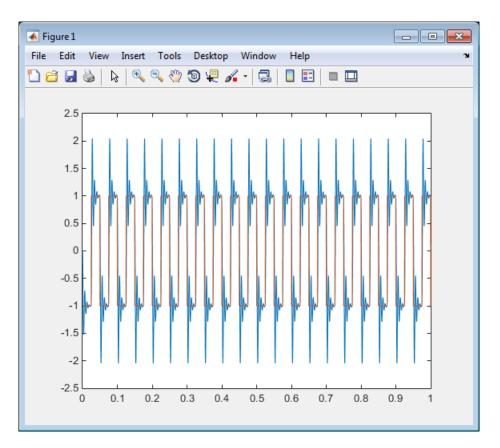
When the real-time application is running in Real-Time mode, data is not saved to the variables tout and yout. Instead, data is saved in the target computer memory and can be retrieved through the target object properties tg.TimeLog, tg.StateLog, and tg.OutLog. However, in the Configuration Parameters dialog box, you must still select the **Time**, **States**, and **Output** check boxes for data to be logged to the target object properties.
