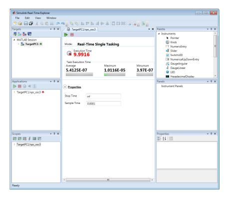
Some blocks cannot handle sample time changes at run-time (see "Blocks Whose Outputs Depend on Inherited Sample Time"). There will be a warning at application build time that changing the sample time might cause incorrect results upon execution. If you see such a warning, change **Fixed step size** in the **Solver** pane of the Configuration Parameters dialog box and rebuild the application.
