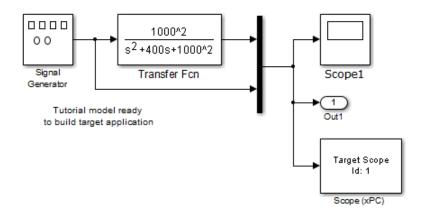
The tutorial shows how to use the Simulink Real-Time software, the Simulink Coder environment, and a third-party compiler. It describes how to create a real-time application from xpc\_osc3, build and download it, and execute it on the target computer.
