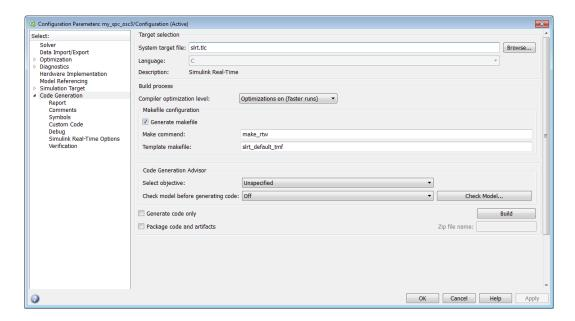
If you have Embedded Coder software, you can build an ERT real-time application. To build an ERT real-time application, in the **Target selection** section, click **Browse** at the **System target file** list. Click slrtert.tlc, and then click **OK**.
